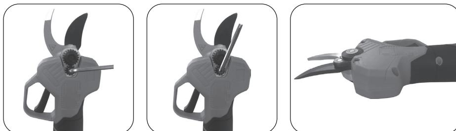
*The fixed and moving blades can be replaced separately; when replacing, there is no need to worry about the opening size of the blade, and the normal opening size will be automatically restored after power on.*
